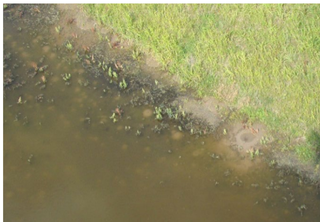
e: Heavy underseepage with sandboil activity
